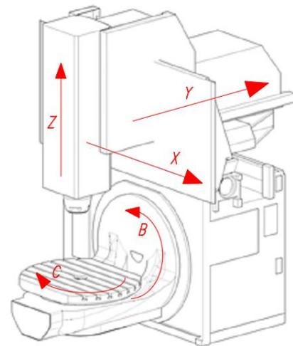
Figure 2. The configuration of Spinner U5-620
