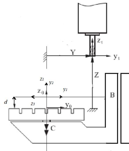
Figure 3. Coordinate systems for Spinner U5-620
