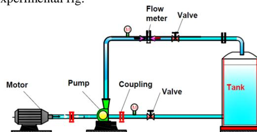
Figure 9. Assembly of experimental rig.
