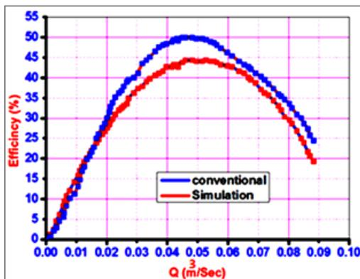
Figure 17. Efficiency comparison between conventional and simulation in (4) blade model
