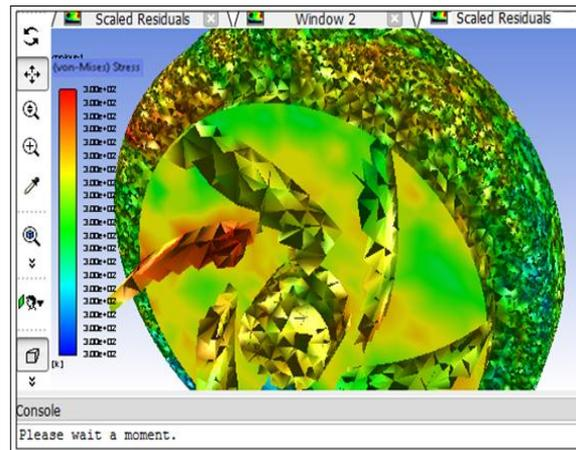
Figure 13. Contours of Von-Mises stresses distributions in six blades.
