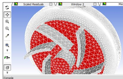
Figure 8. Six Impellers after mesh smoothing.
