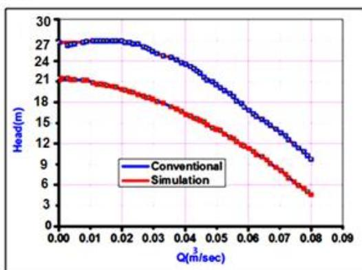
Figure 18. Head comparison between conventional and simulation in (6) blade model.
