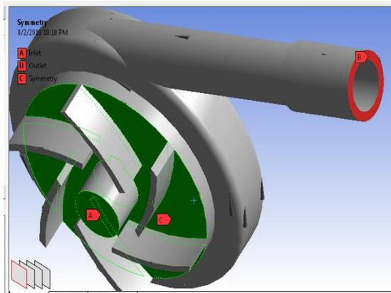
Figure 4. Boundary condition in blade impeller.
