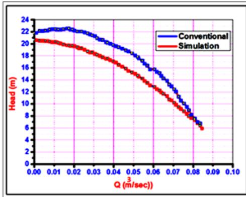
Figure 16. Head comparison between conventional and simulation in (4) blade model.
