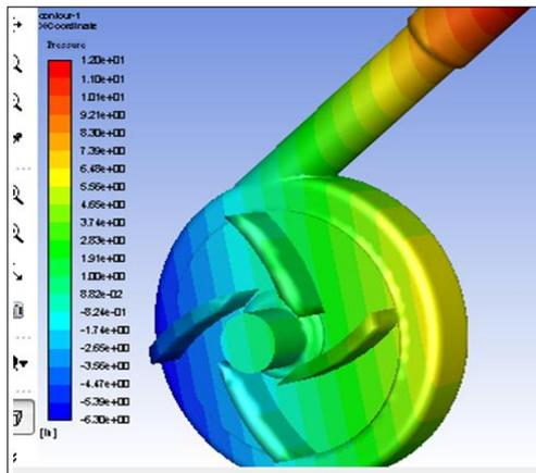
Figure 10. Pressure contours (4) blades impeller.
