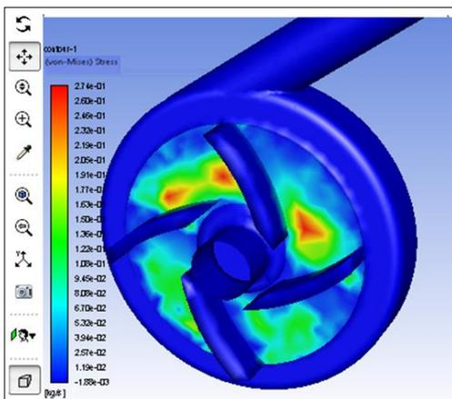
Figure 12. Contours of Von-Mises stresses distributions in 4 blades.
