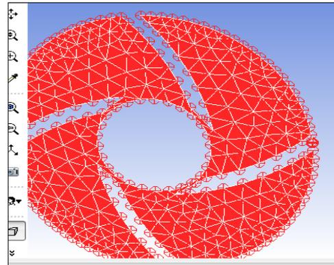
Figure 7. Four Impellers after mesh smoothing.
