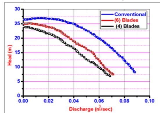
Figure 20. Comparison between heads values of conventional and simulation.
