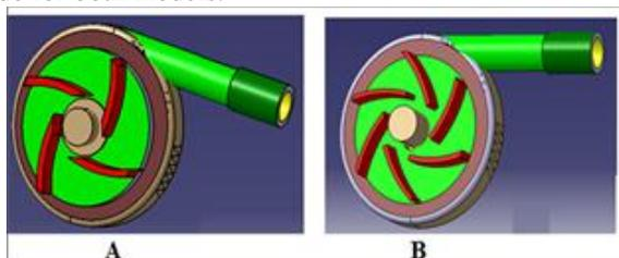
Figure 3. (A) Assembly of four blades, (B) Assembly of six blades model.
