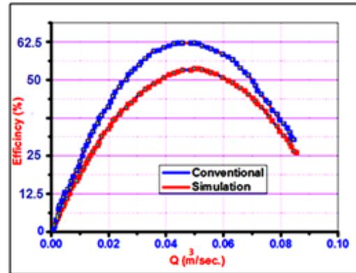
Figure 19. Efficiency comparison between conventional and simulation in (6) blade model.
