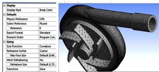
Figure 6. Mesh (6) blades impeller.
