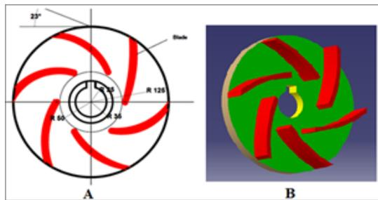
Figure 2. (2D) and (3D) for second impeller model.
