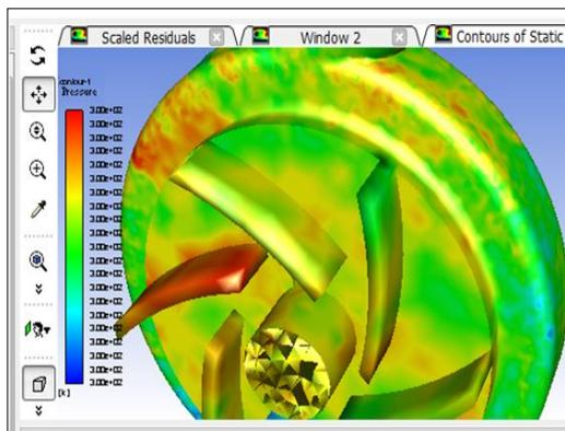
Figure 11. Pressure contours (6) blades impeller.
