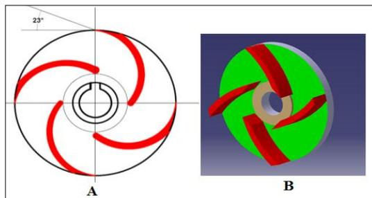
Figure 1. (2D) and (3D) for first impeller model.
