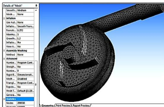
Figure 5. Mesh (4) blades impeller
