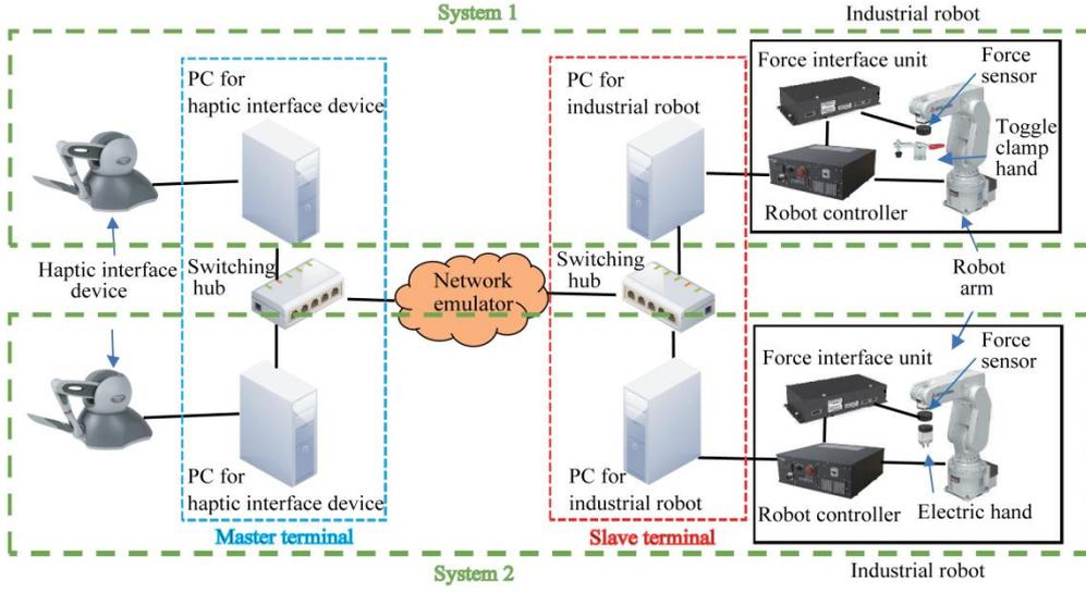
Figure 1. Configuration of two remote robot systems with force feedback in assessment.
