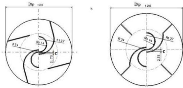
Figure 2. Combined of Savonius tandem blade with tangential and radial moving plate deflector [4].
