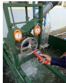
Figure 7. Measuring torque and shaft revolution.
