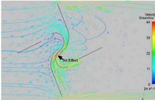
Figure 3. Jet Effect phenomena on the concave blade by using combined STB and Tangential MPD [4].
