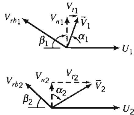
Figure 5. Inlet velocity polygons and outlet velocity polygon.
