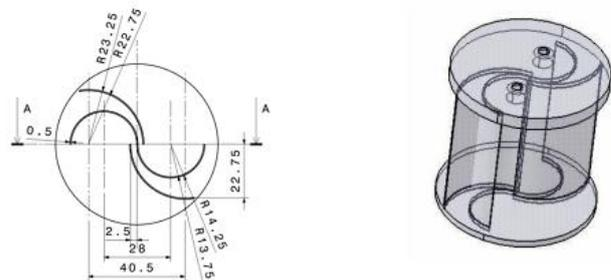
Figure 1 Design of Savonius Tandem Blade (STB) [4].
