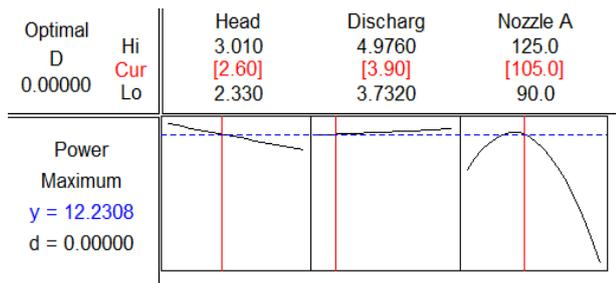
Figure 9. Power maximum at position 2.60 [m], 3.90 [lt/s] and 105[°].
