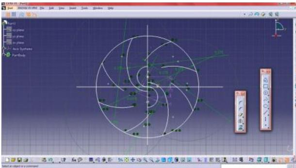
Figure 4. New cross flow runner design with Savonius tandem blade using CAD software (Catia).
