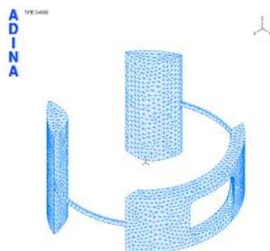
Figure 3. Structural analysis model of air chambers
