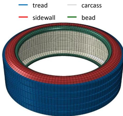
Figure 2. Finite element model of simplified tires.
