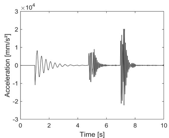
Figure 8. The acceleration result of the quarter vehicle.
