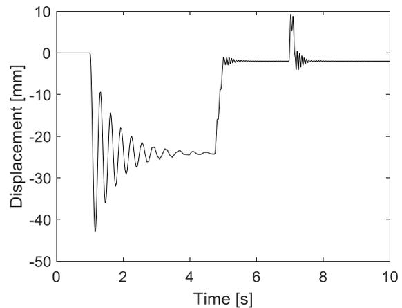
Figure 7. The displacement result of the quarter vehicle.
