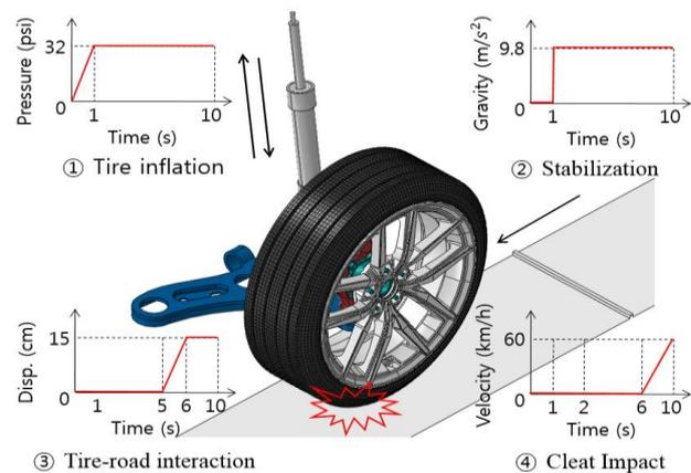
Figure 3. Boundary conditions of the cleat impact analysis.
