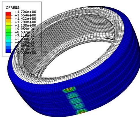
Figure 5. The contact pressure distribution of the tire.
