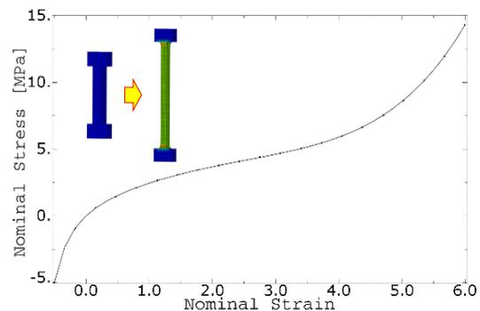
Figure 1. Nominal stress-strain relationship curve for the hyper-elastic materials from Yeoh model coefficients.
