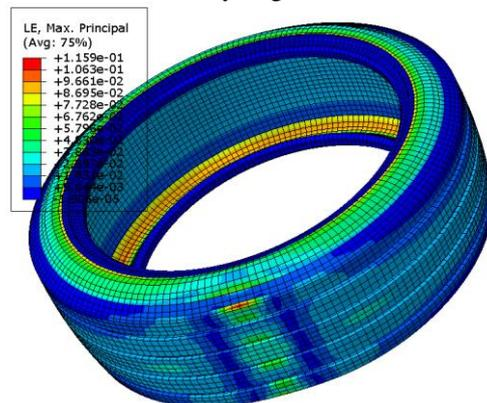
Figure 4. The strain of the tire.
