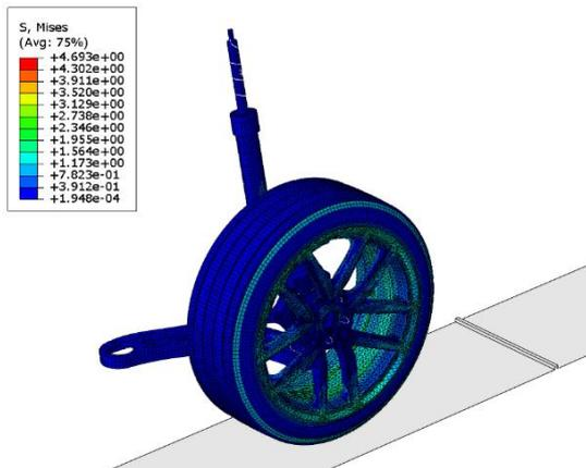
Figure 6. The stress result of the quarter vehicle.
