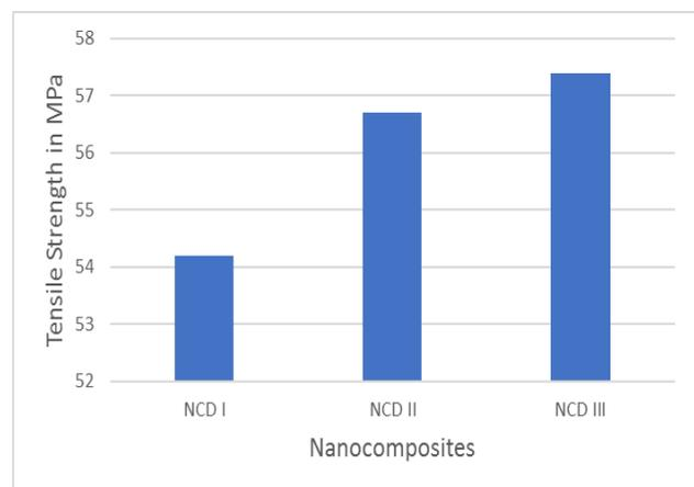
Figure 1. Tensile strength of NCD.
