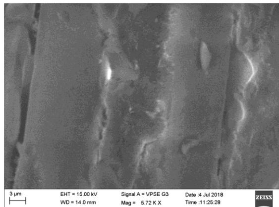
(e) Interphase of glass fiber and nanoclay-epoxy
