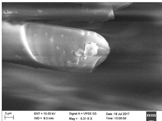
(b) Rupture and pulling out of the glass fiber
