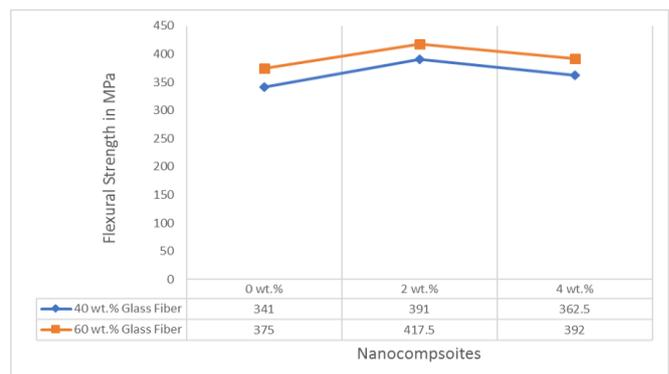
Figure 4. Flexural strength of NCF.
