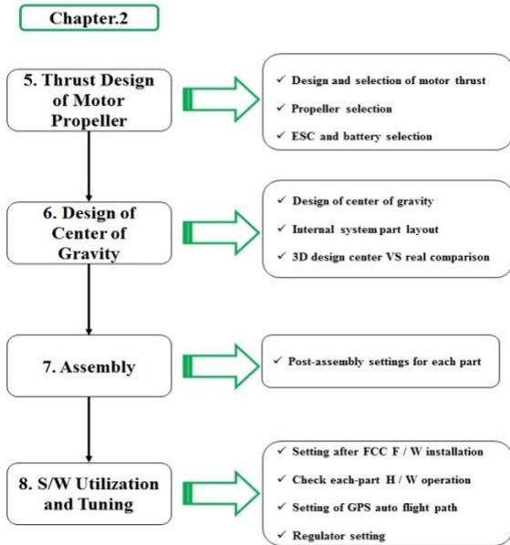
Figure 3. Development process of UAV Chapter 2
