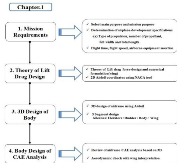
Figure 2. Development process of UAV Chapter 1
