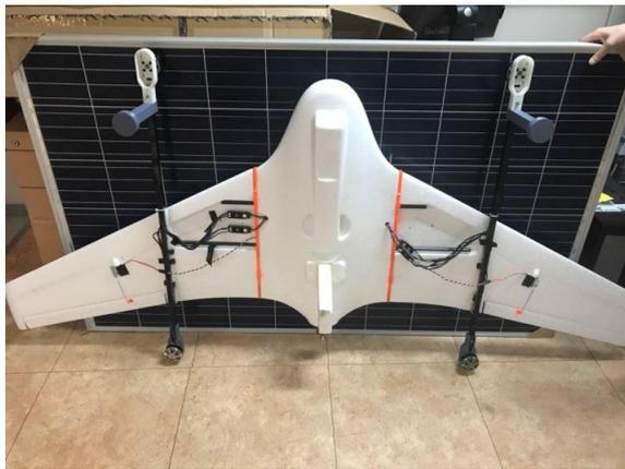
Figure 16. Airframe attached with carbon fiber columns
