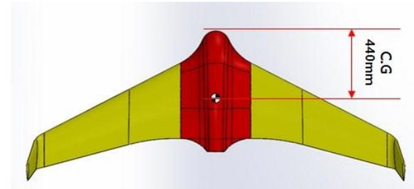
Figure 13. Center of gravity
