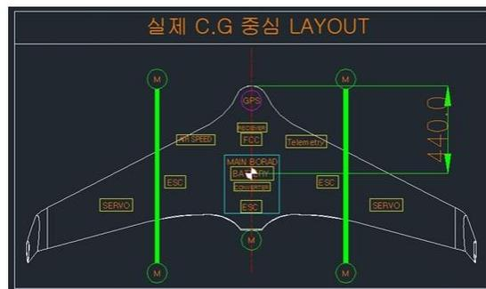
Figure 14. Product module relocation LAYOUT
