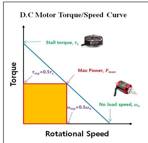
Figure 11. Motor torque / speed curve plot
