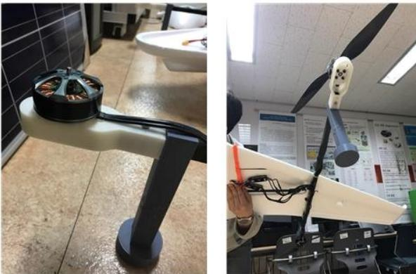
Figure 17. Floor support made with 3D printer
