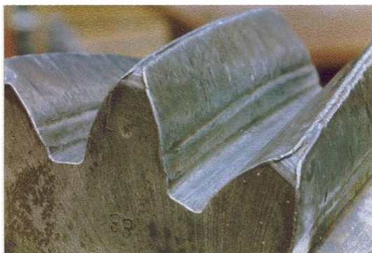
Figure 1. The example abrasion the details of the mechanism.
