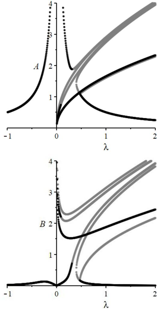
Figure 4. The amplitude-frequency characteristics of the forced stationary oscillations when  $v_1=0.1$ .
