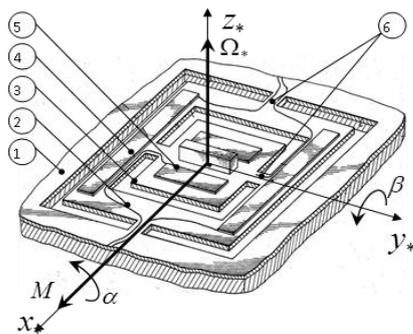
Figure 1. Micromechanical gyroscope RR-type.
