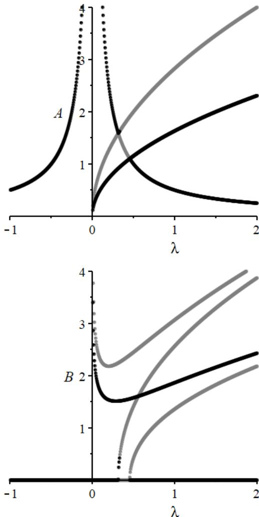
Figure 3. The amplitude-frequency characteristics of the forced stationary oscillations when  $v_1=0$ .
