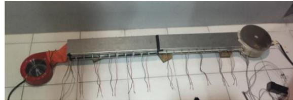
Figure 2. Fabricated heat exchanger device
