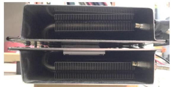
Figure 3. Cross sectional representation of heat exchanger device
