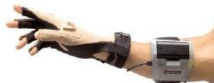
Figure 2. Cyberglove II flex sensors based MCS (Cyberglove Systems image)
