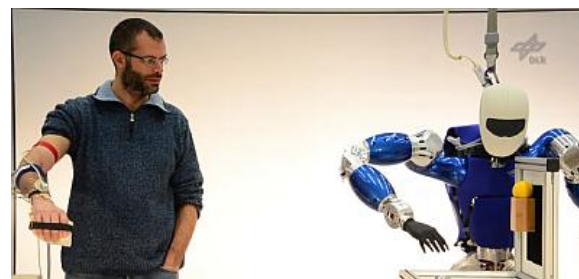
Figure 3. Robot torso controlled by EMG signals (DLR photo)
