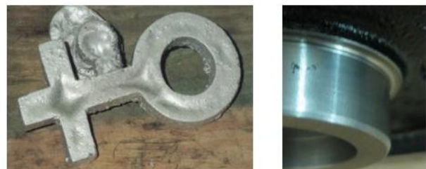
Figure 2. Example of defect by shrinkage
