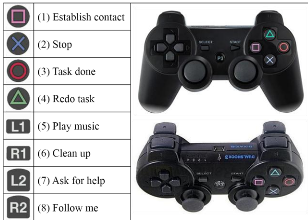
Figure 2. Command list and wireless joystick for teleoperation.
