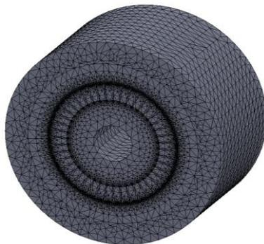
Figure 5. The 3-D mesh of induction motor
