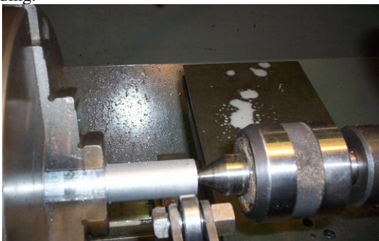
Figure 1. Setup of burnishing experiments as conducted on a lathe machine
