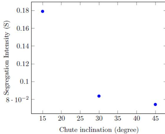
Figure 12. Segregation Intensity of particles in an inclined chute
