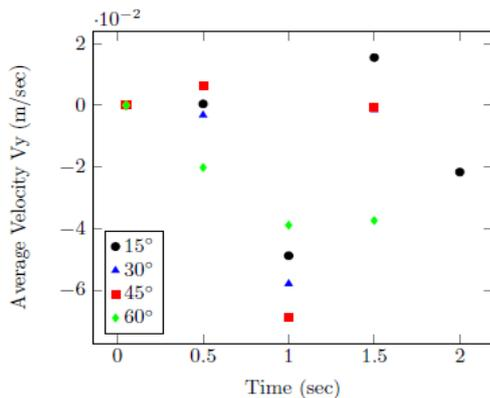
Figure 6. Average velocity of particles in y-direction in an inclined chute
