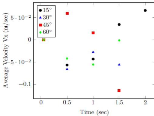
Figure 5. Average velocity of particles in x-direction in an inclined chute
