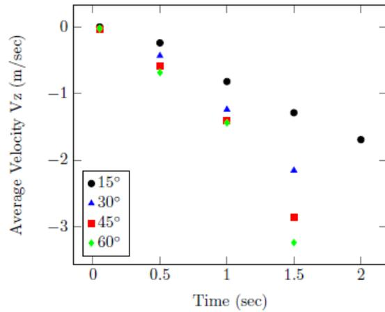
Figure 7. Average velocity of particles in z-direction in an inclined chute
