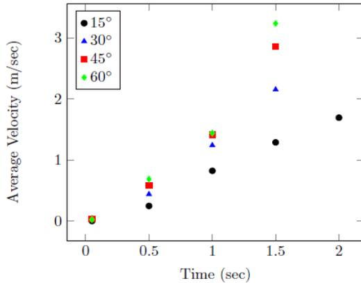
Figure 4. Average velocity of particles in inclined chute over time for different inclination angles
