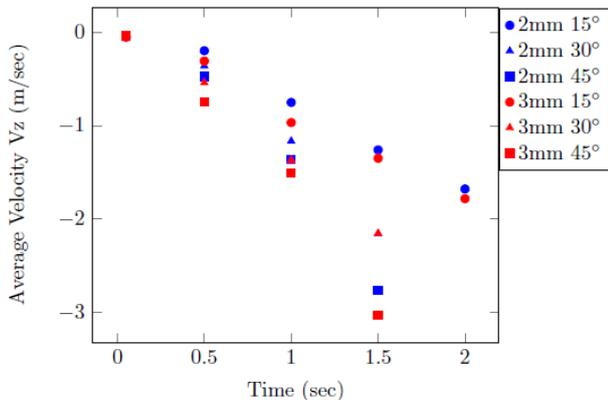
Figure 10. Average velocity of different particles in particles in x-direction in an inclined chute
