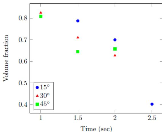
Figure 11. Volume fraction of larger particles in an inclined chute
