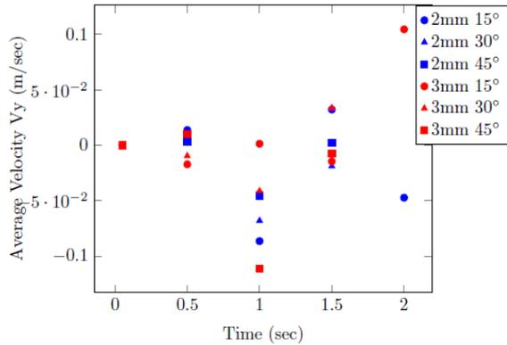
Figure 9. Average velocity of different particles in y-direction in an inclined chute
