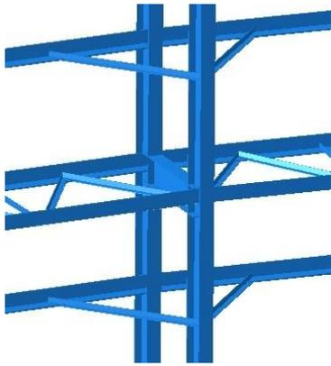
Figure 11. Tied joint of members in circumferential bracing system
