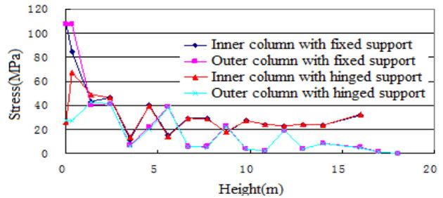
Figure 10. Stress curves with height of a vertical rigid frame
