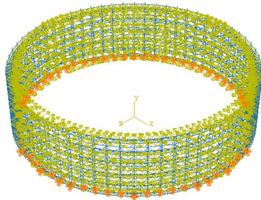
Figure 6. Retaining frame model with load and boundary constraint.
