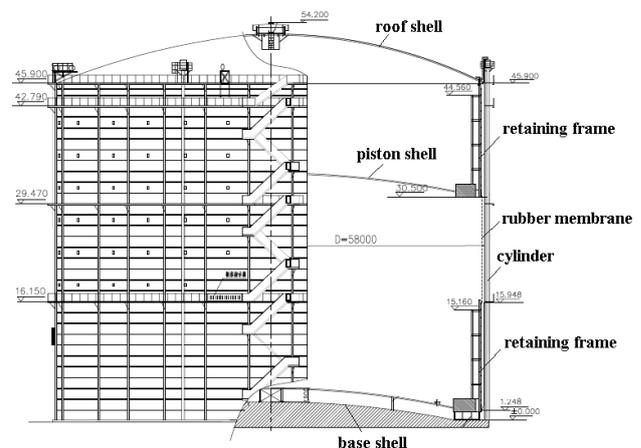
Figure 2. Structural sketch of one-stage gasholder.
