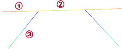
Figure 13. Member number of horizontal knee bracing
