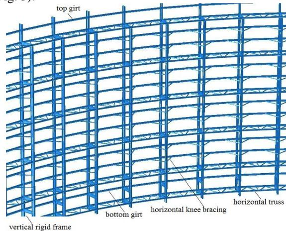
Figure 5. Partial model of piston retaining frame.
