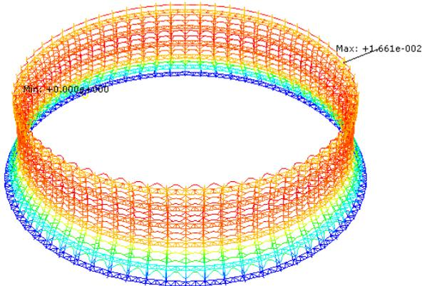
Figure 7. Deformation diagram of retaining frame.
