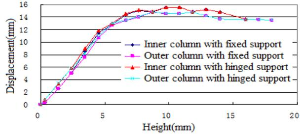
Figure 9. Displacement curves with height of a vertical rigid frame
