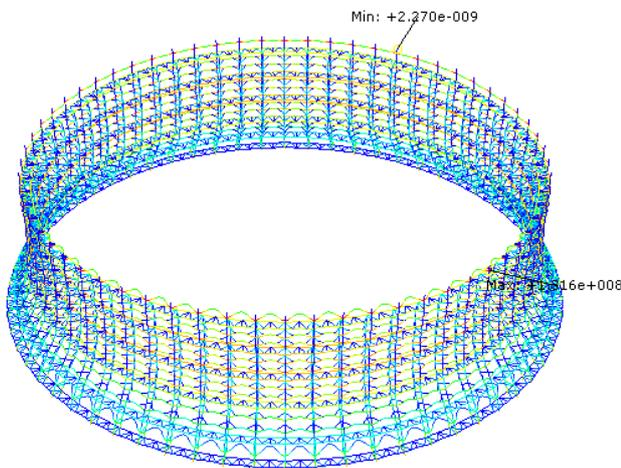
Figure 8. Mises stress diagram of retaining frame.
