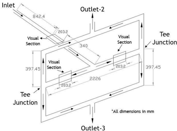
Figure 1b. Details of the test-section
