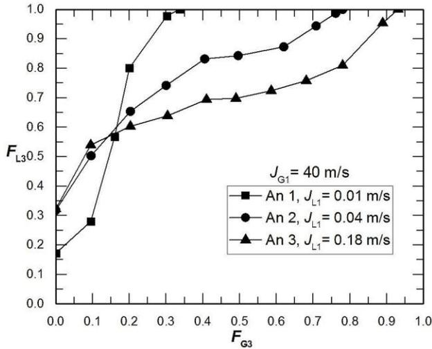
Figure 3. Effect of  $J_{L1}$  on partial-phase separation with two vertical impacting tees.
