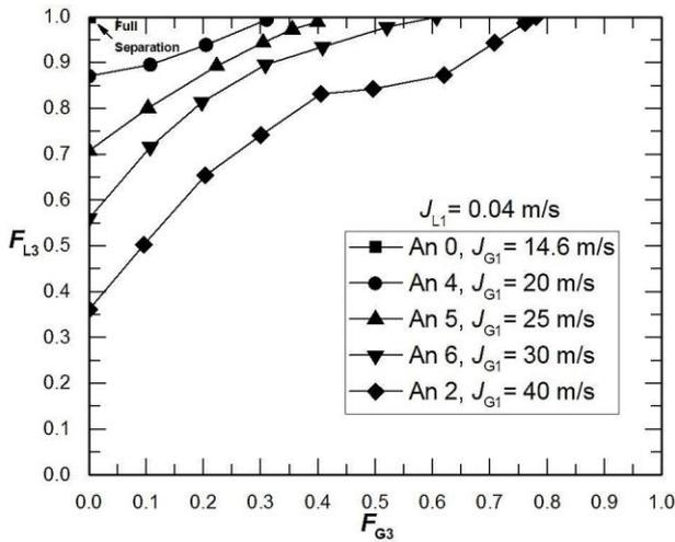
Figure 4. Effect of  $J_{G1}$  on partial-phase separation with two vertical impacting tees.
