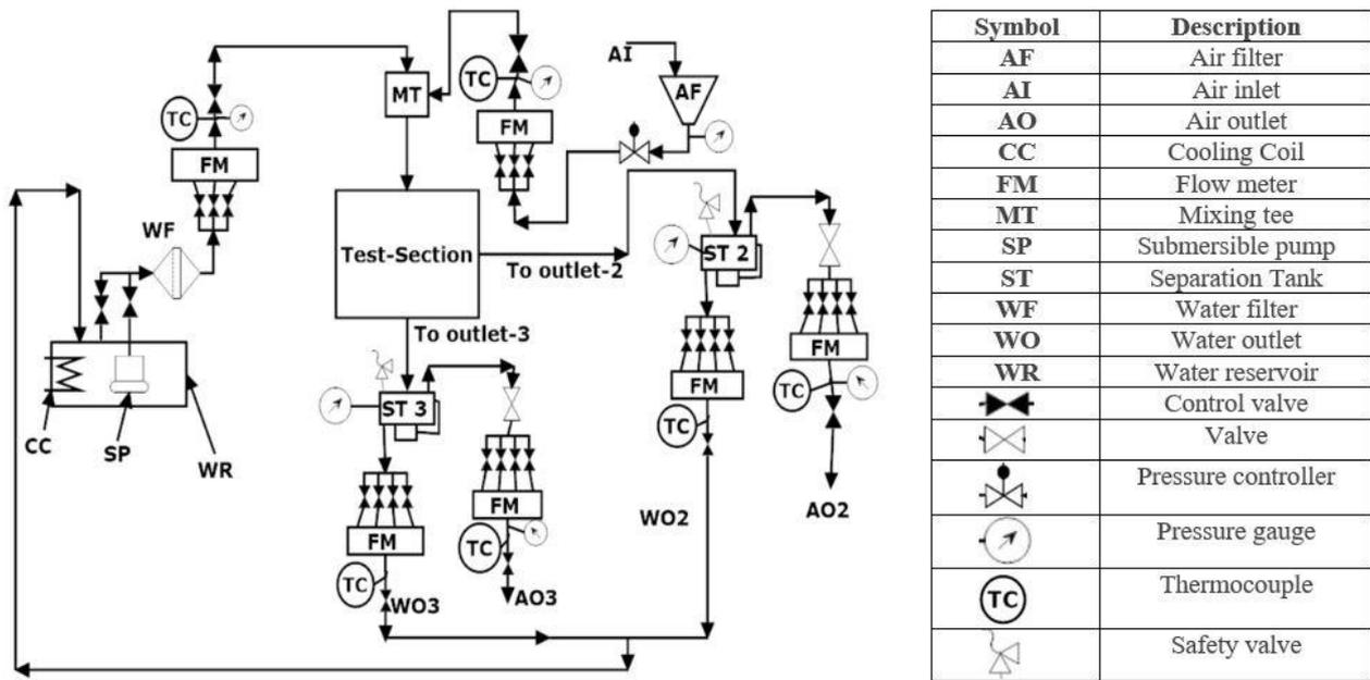
Figure 1a. Schematic diagram of the test loop.
