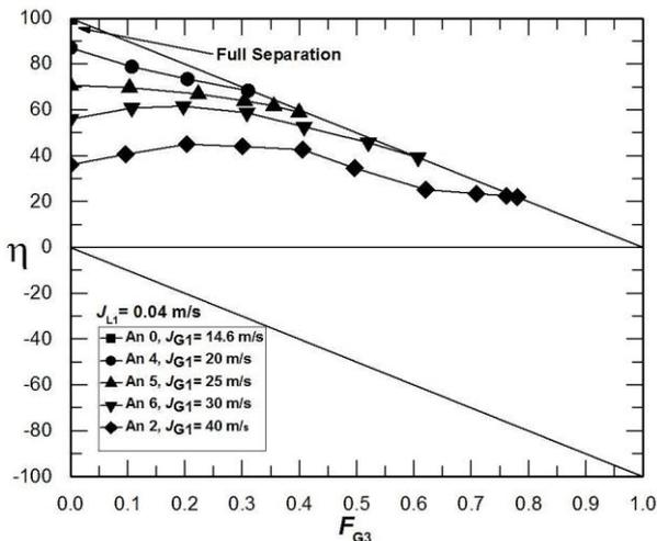
Figure 9. Effect of  $J_{G1}$  on phase-separation parameter with two vertical impacting tees.
