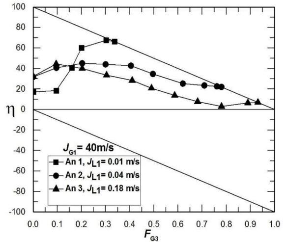
Figure 10. Effect of  $J_{L1}$  on phase-separation parameter with two vertical impacting tees.
