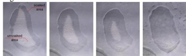
Figure 6. Increase of wetted area over time inside transparent battery cell.
