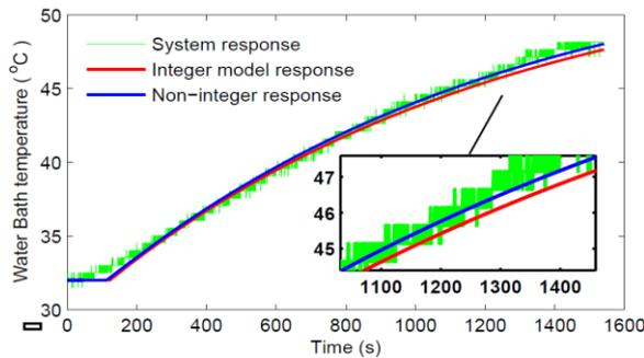
Figure 8. Open Loop Step Responses for Water Bath System
