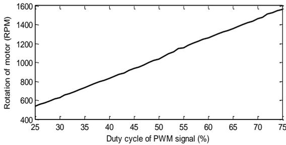
Figure 4. Input output steady state characteristics for DC motor
