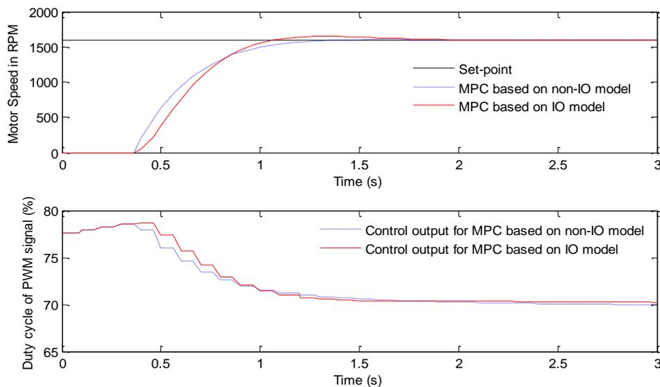
Figure 10. Closed loop Step response for DC motor system
