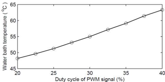
Figure 5. Open loop input-output characteristic of Water Bath system
