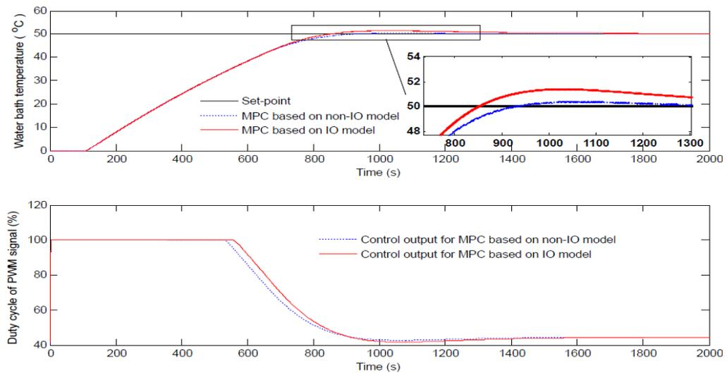
Figure 13. Closed loop Step response for Water Bath system
