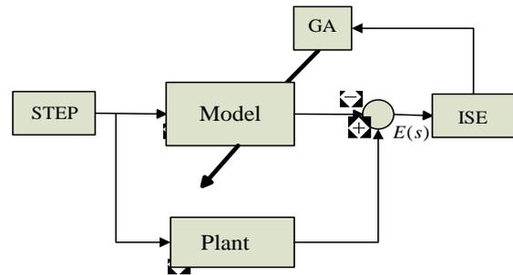
Figure 6. GA optimized Model Parameters
