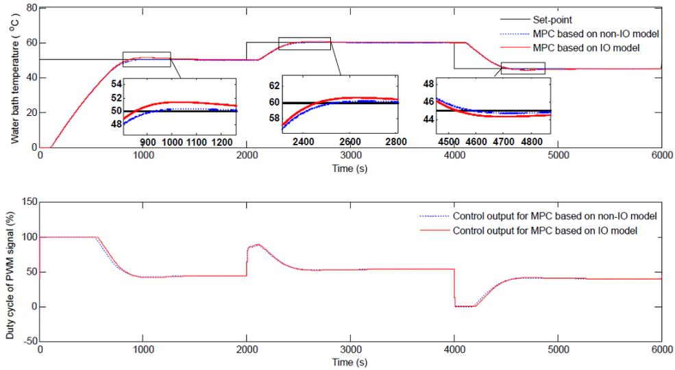
Figure 14. Closed loop Servo Response for Water Bath system
