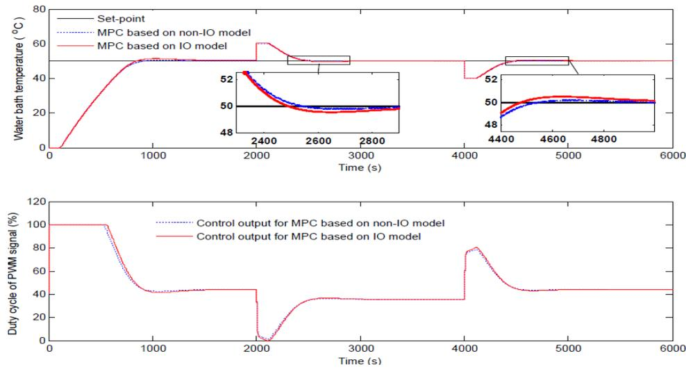
Figure 15. Closed loop Regulatory Response for Water Bath system
