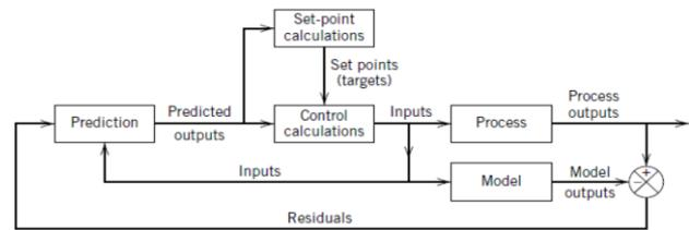
Figure 9. MPC Structure
