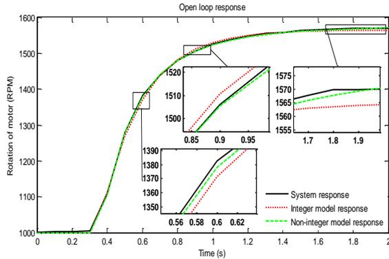
Figure 7. Open Loop Step Responses for DC motor
