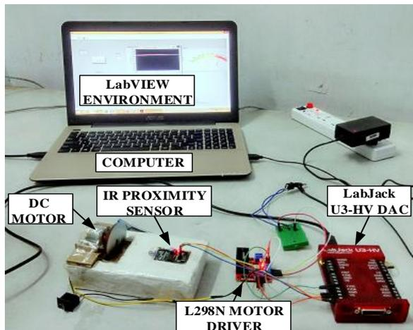
Figure 2. DC motor speed control system
