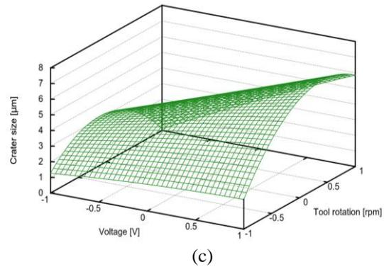
Figure 4. Response surface plot of crater size (a) combined effect of voltage and capacitance (b) combined effect of tool rotation and capacitance (c) combined effect of voltage and tool rotation.
