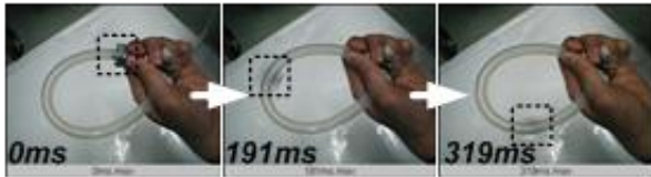
Figure 2. Movement of flexible pneumatic cylinder.
