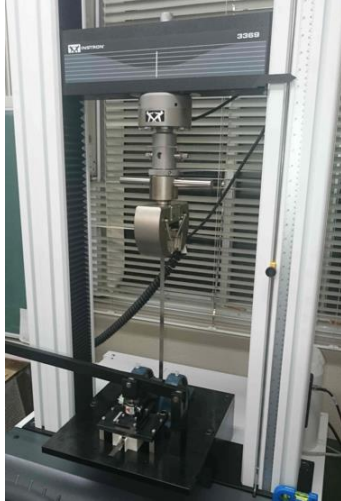
Figure 2. Tensile testing machine (Tolerable load: 50kN) and friction test apparatus.
