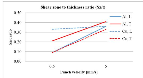
Figure 7. Ratio of Sz/t to the v1 and v2
