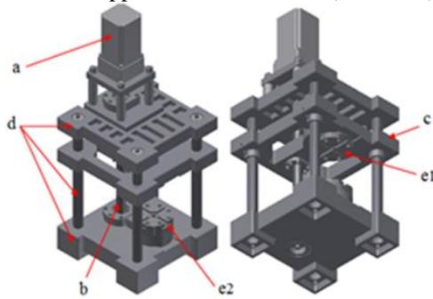
Figure 1. 3D model and detailed drawing of  $\mu$ -Forming machine 5kN. Sub-Function of micro forming machine; a). Servo motor, b). Ball screw, c). ram, d). Frame and guiding set, e). Bolster.
