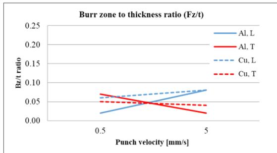
Figure 9. Ratio of Bz/t to the v1 and v2
