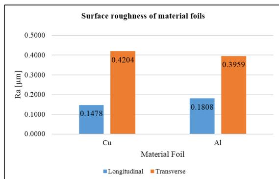
Figure 3. Material foils surface roughness
