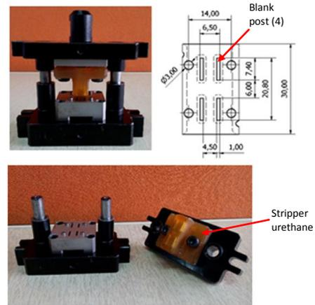
Figure 2. Micro blanking tool.
