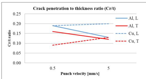
Figure 10. Ratio of Cr/t to the v1 and v2
