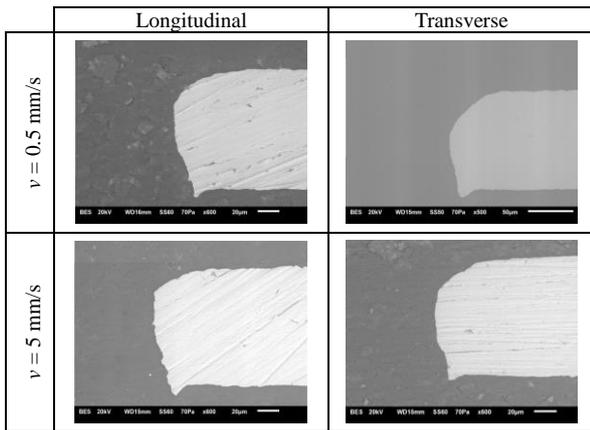
TABLE IX. SHEAR EDGE PORTION OF ALUMINUM BLANKING PART
