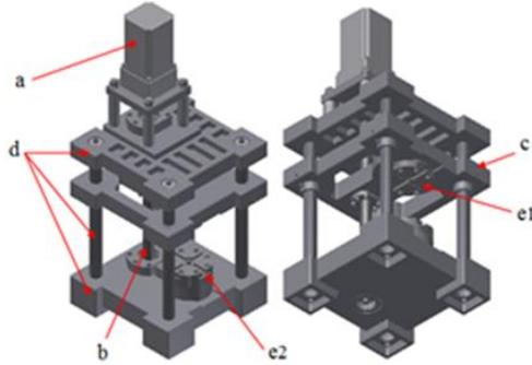
Figure 1. 3D model and detailed drawing of μ-Forming machine 5kN. Sub-Function of micro forming machine; a). Servo motor, b). Ball screw, c). ram, d). Frame and guiding set, e). Bolster.
