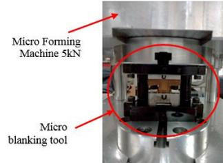
Figure 4. Mounted micro-blanking tool
