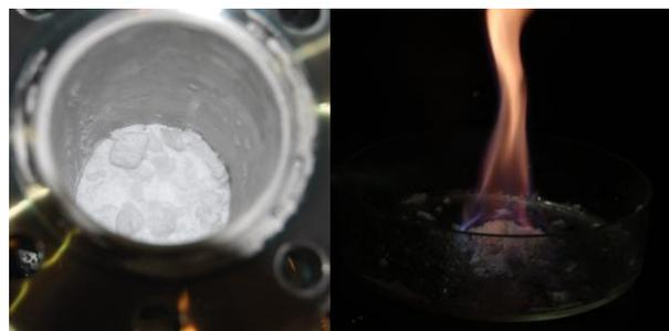
Figure 4. Methane hydrate synthesized in this experiment. (Left: Methane hydrate, Right: Combustion of methane hydrate).
