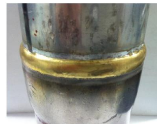
Figure 9. Arc brazing applied joining of muffler part
