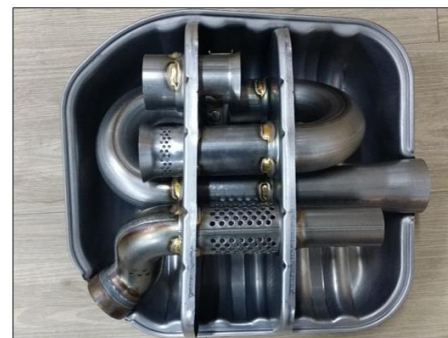
Figure 10. Case study of arc brazing process for internal part of main muffler for minimum welding distortion
