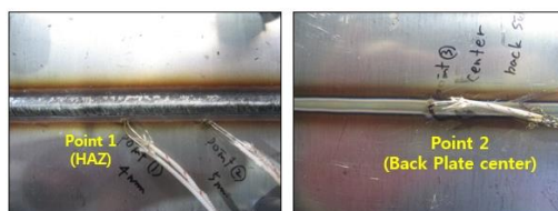
Figure 2. Location of thermocouple attached on HAZ and back plate of center
