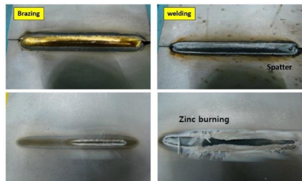
Figure 4. Comparison of zinc burning phenomenon
