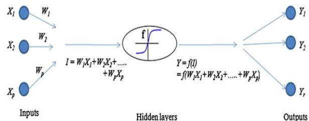
Figure 1. Artificial neural network model
