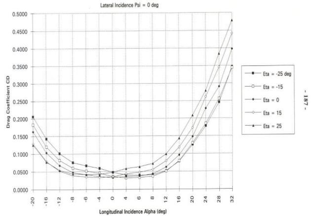
Figure 2. Aerodynamic data for coefficient of drag expressed as a function of angle of attack, roll angle and elevator deflection angle
