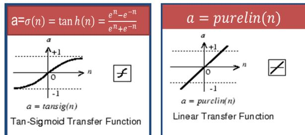
Figure 3. Tan-Sigmoid and linear transfer function
