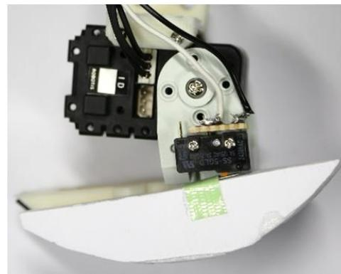
Figure 5. A Touch sensor on the foot
