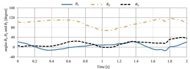
Figure 9. Temporal dynamics of the joints' angles for the robot walking with P control
