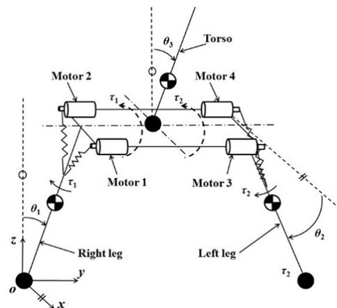
Figure 1. The model of the biped walking robot with antagonistic actuation
