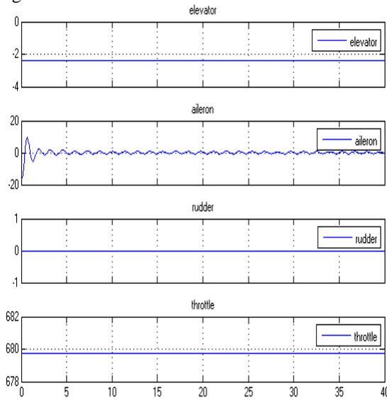
Figure 7. Changes of elevator, aileron, rudder and throttle as results of the applied controller.
