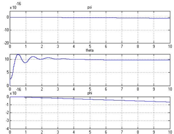
Figure 5. Changes of psi, theta and phi as results of the applied controller.
