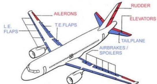
Figure 1. Flight control surfaces on airliner [6].
