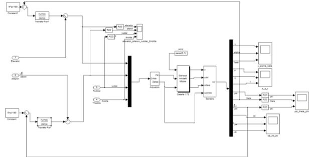
Figure 9. The simulink model for MIMO system
