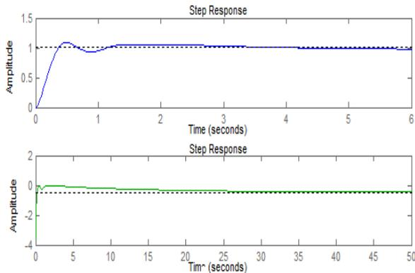
Figure 3. Theta output and elevator input step responses for the PID controller
