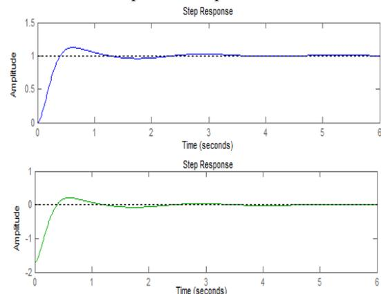
Figure 6. Phi output and aileron input step responses for the PID controller
