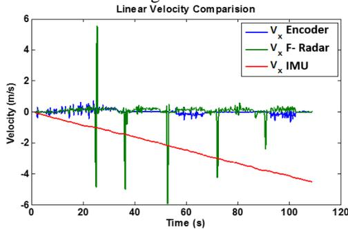
Figure 4. The comparison of linear velocities from the encoder, FMCW Radar and inertial measurement unit (IMU)
