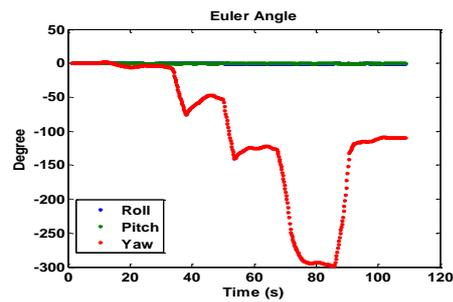
Figure 7. Euler angles of roll, pitch, and yaw from IMU
