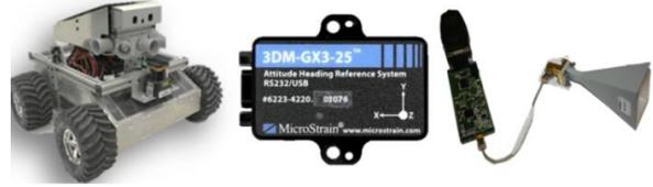
Figure 1. Mobile robot platform (left), inertial measurement unit (center), and FMCW radar (right)
