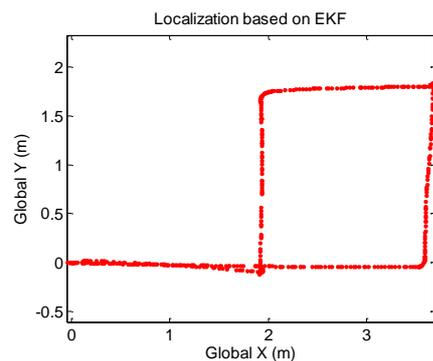
Figure 8. The localization results of the mobile robot
