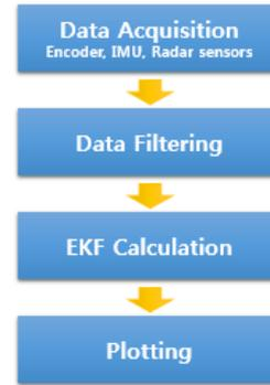
Figure 3. The flow chart for EKF in Matlab code
