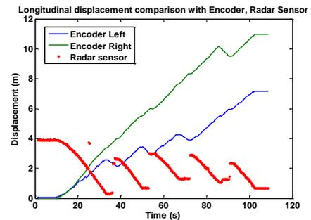
Figure 6. Displacement of both encoders and FMCW Radar
