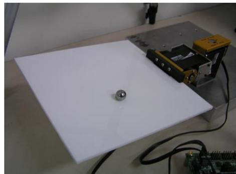
Figure 1. The ball-plate system studied in this paper.
