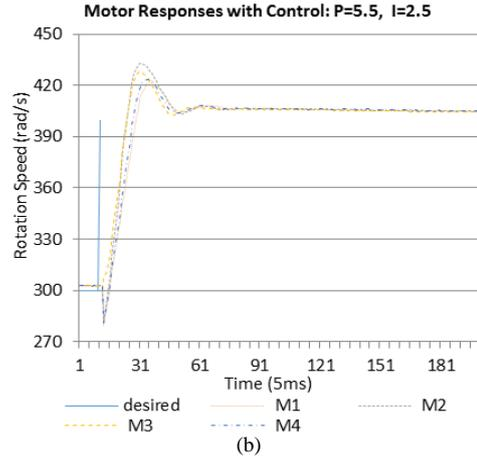
Figure 4. Response of motors from 300 rad/s to 400 rad/s
