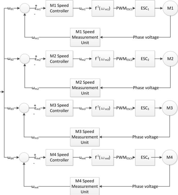
Figure 2. Block diagram of hierarchical control
