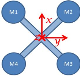
Figure 1. Simplified schematic diagram of a quadcopter in Cross-Configuration
