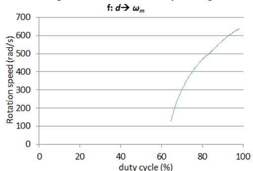
Figure 3. Plotting rotation speed of motor against duty cycle of PWM of ESC
