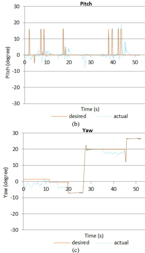
Figure 6. Attitudes in flights with cascaded motor control and attitude control
