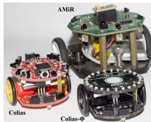
Figure 1. Colias- $\Phi$ , Colias and AMiR mobile robots developed for swarm robotic applications
