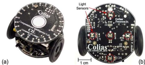
Figure 2. Colias- $\Phi$  micro robot platform developed for pheromone communication system
