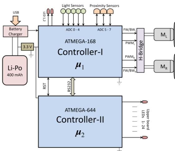
Figure 3. Architecture of Colias- $\Phi$
