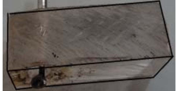
Figure 9: Perspex and Tool Burning by Type-I Drill Bit
