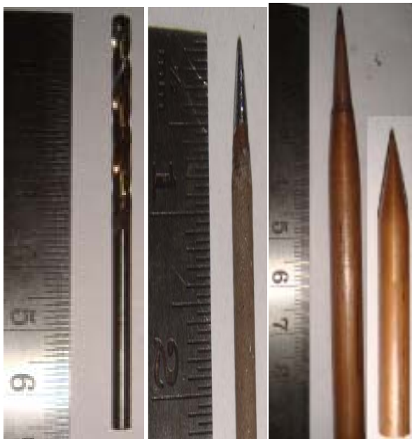
Figure 4: (a) Steel Grooved (Type-III), (b) Mild Steel Coated (Type-IV), and (c) Copper Tapered (Shorter Length: Type-Va, Longer Length: Type-Vb) Drill Bits
