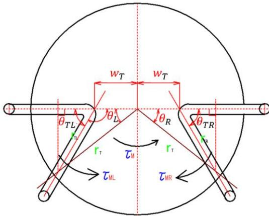
Figure 2. Improved servo valve using buckled tube.
