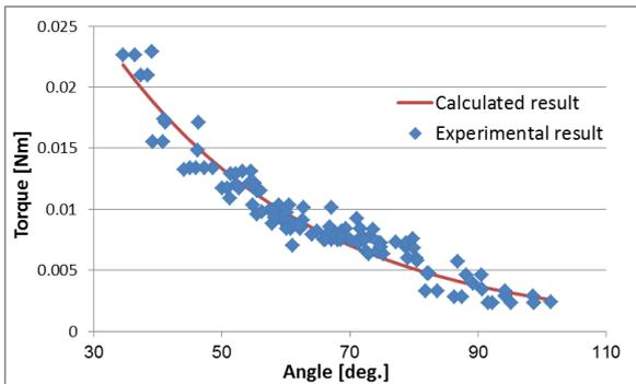
Figure 3. Relation between buckled angle and restoration torque
