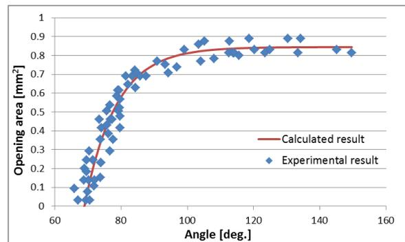
Figure 5. Relation between buckled angle and opening area
