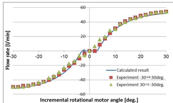
Figure 6. Relation between buckled angle and mass flow rate
