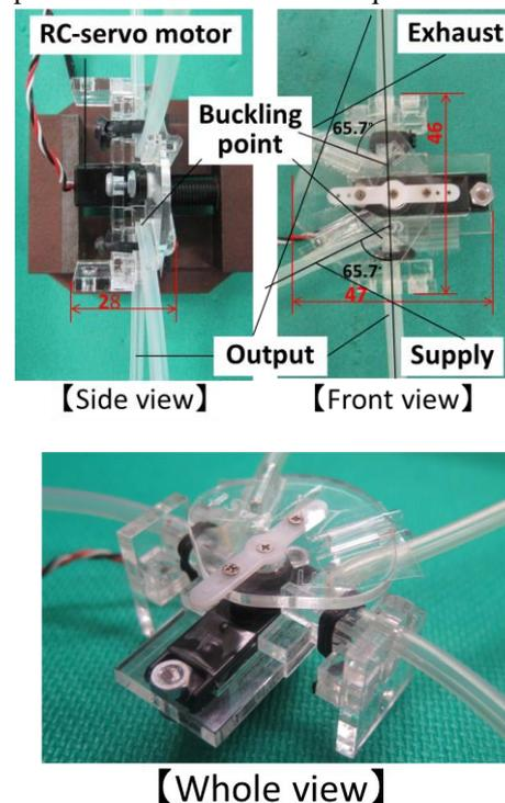
Figure 1. Improved servo valve using buckled tube.
