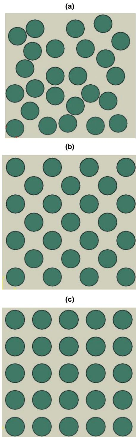
generated each measuring 133 x 133 m containing 25 complete fibers with 18m diameter as shown in Figure 1.
