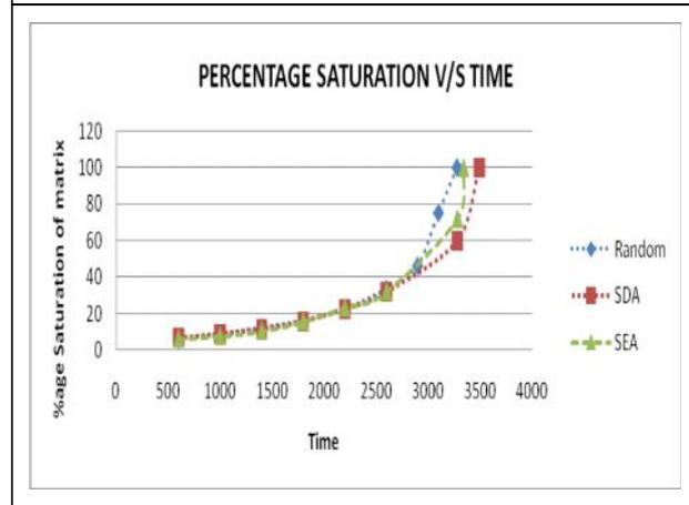
Time taken for entire epoxy to fully saturate was 3280, 3495, 3340 sec for RA, SDA and SEA arrangements respectively. The rate of heat transfer through different fiber topologies have been shown in Figure 4 which gives a comparison between differences in rate of heat transfer.
