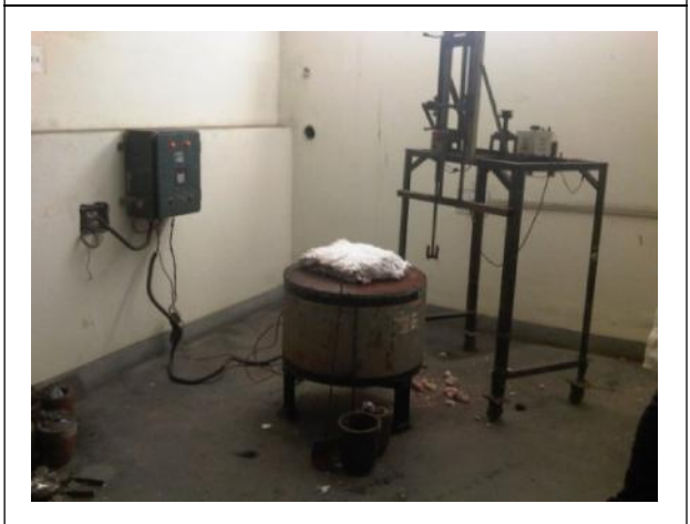
Figure 1: Furnace with Stirring Apparatus
