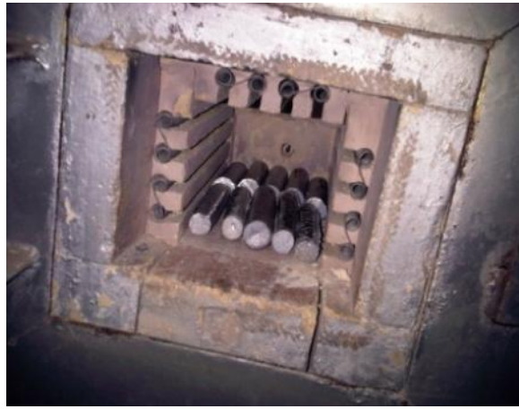
Figure 2: Heat Treatment in Muffle Furnace
