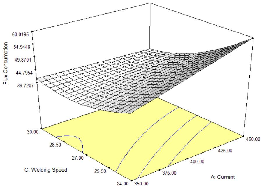
**Figure 4: 3D Surface Graphs for the Flux Consumption Between Voltage and Current**
