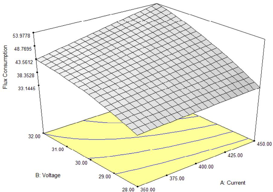
**Figure 5: 3D Surface Graphs for the Flux Consumption Between Welding Speed and Voltage**
