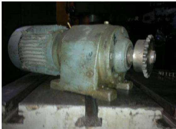
Specification of driving gearbox. Reduction ratio 1500 to 80 rpm.
