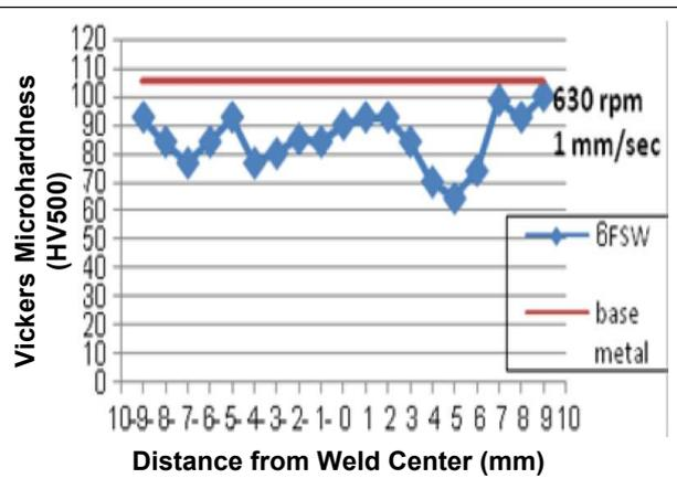
**Figure 34: Microhardness Profile in Welded Joint/FSW7**
