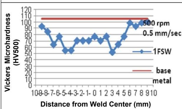
**Figure 31: Microhardness Profile in Welded Joint/FSW2**
