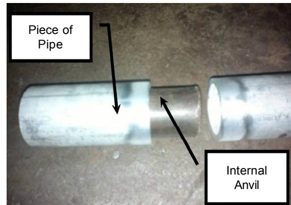
**Figure 4: Fixing Mandrel**
