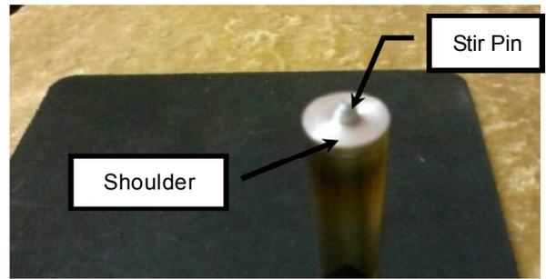
a mixture of frictional heating and forging pressure, most of heat generation related to the tool shoulder while the probe When descended to the part, the rotating pin contacts the surface producing frictional heating which softens a small column of metal.
