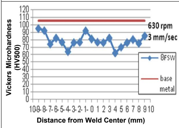
**Figure 38: Microhardness Profile in Welded Joint/FSW11**
