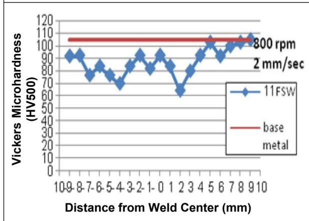
**Figure 36: Microhardness Profile in Welded Joint/FSW9**
