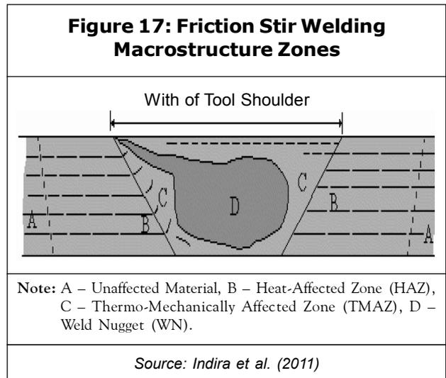
grains are found in the nugget zone, in contrast to the TMAZ and HAZ zones where coarsened grains are observed (Soundararajan *et al.*, 2006).
