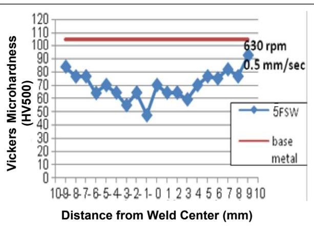
**Figure 33: Microhardness Profile in Welded Joint/FSW6**
