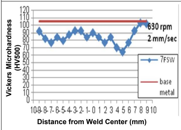
**Figure 37: Microhardness Profile in Welded Joint/FSW10**
