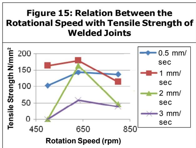
with different welding speed (0.5, 1, 2, 3 mm/sec) and from above results we see increasing in tensile strength with increase the welding speed from 0.5 to 1 mm/sec but when increasing the welding speed to 2 and 3 mm/s the tensile properties of the joints seriously deteriorate and reach to minimum value 38.25 mpa for welding speed 3 mm/s with 800 rpm, joint efficiency 13.18.
