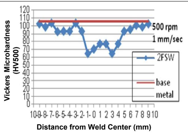
**Figure 32: Microhardness Profile in Welded Joint/FSW5**
