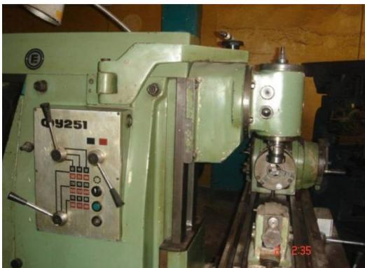
The milling machine used has rotational speed on the head that is suitable to fixing welding tool on it, but it has linear speed on table that is not match with the objective of the study (need circular rotational feed) so that some apparatus were adapted on its working table. Figure 2 shows schematically Friction Stir Welding (FSW) apparatus and equipments.
