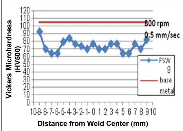
**Figure 39: Microhardness Profile in Welded Joint/FSW12**
