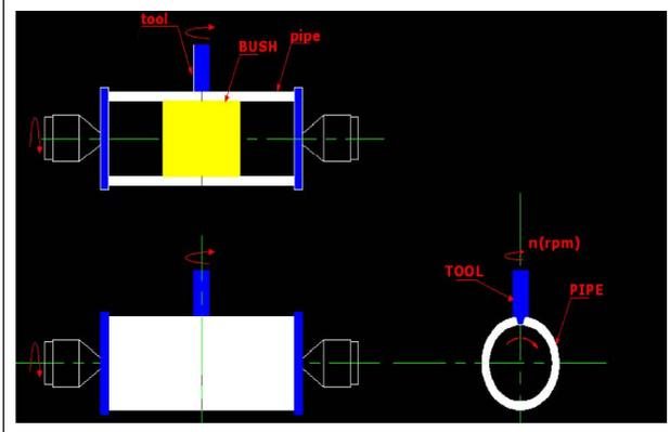
A rotating clamping fixture where designed to clamps and hold the two segments of pipe together for butt joint welding.
