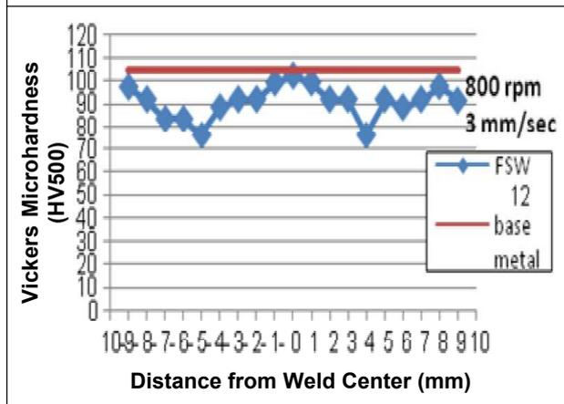
(advancing side) for the rotating tool where the rotational velocity vector and the forward motion vector are in the same direction and due to this there is higher heating on one side of the weld center and hence lower hardens.
