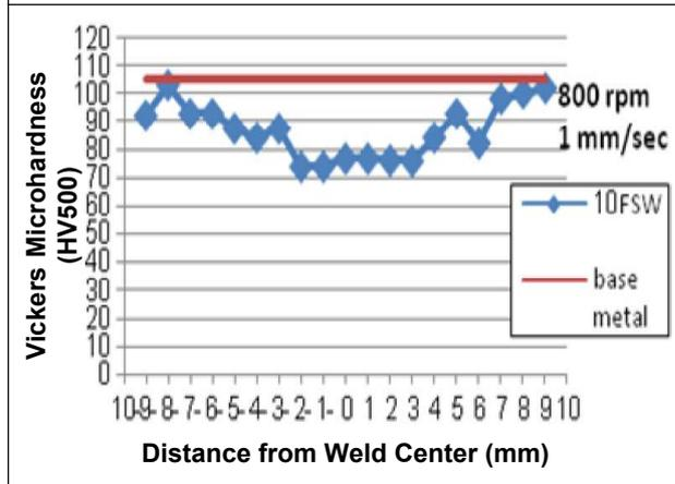
**Figure 35: Microhardness Profile in Welded Joint/FSW8**
