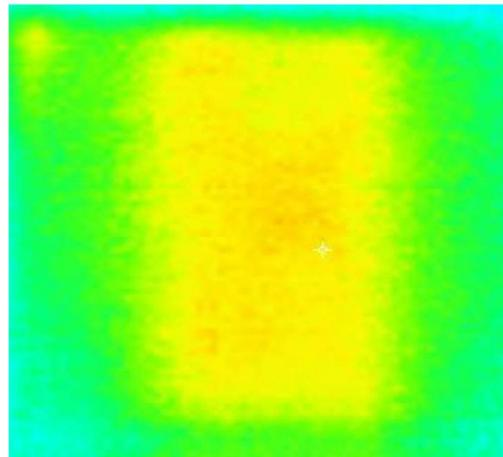
c) Sample 3 (Delamination Beneath Four Layers with Depth 1.25 mm)
