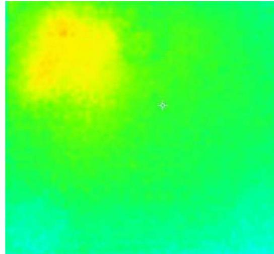
**b) Sample 2 (Circular Delamination with Thickness 0.1 mm)**
