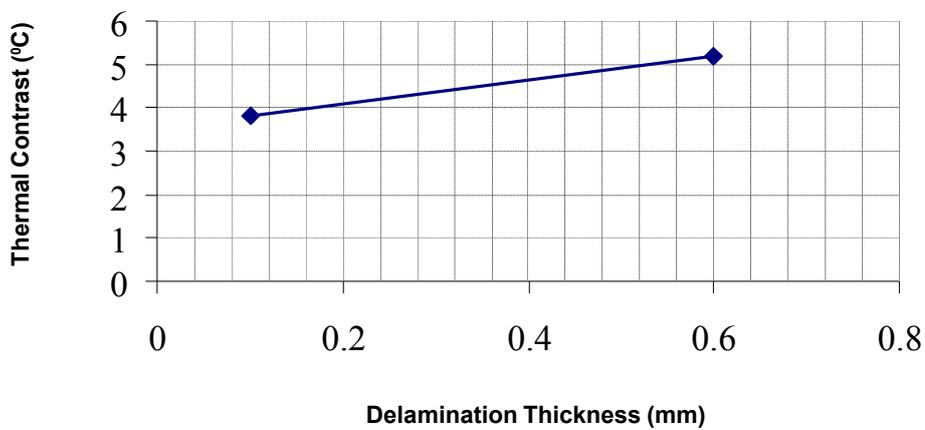
Due to the difference in thermal resistance of delamination, the thermal contrast values obtained were 5.2 °C and 3.8 °C, for sample 1 and 2 respectively. As the thickness of delamination increases the thermal resistance of the delamination is increases. This results in higher thermal contrast at the location of thicker delamination.
