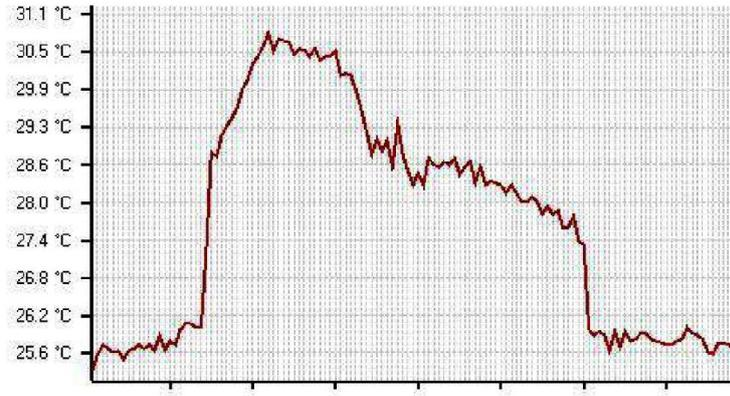
**b) Temperature Profile of Sample 2 (Delamination Thickness 0.1 mm)**
