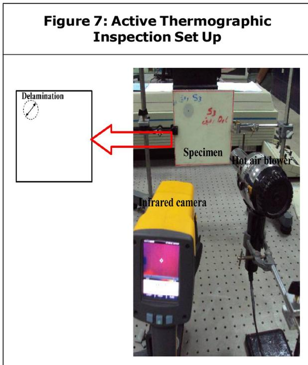
**Figure 7: Active Thermographic Inspection Set Up**
