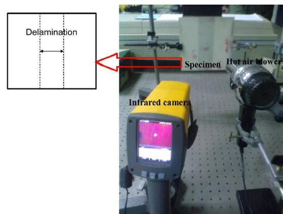
Fluke Ti20 infrared camera. It has an un-cooled detector with focal plane array 128X96HV, where infrared detector absorbs the infrared energy emitted by the studied specimens and converts it into electrical signal.
