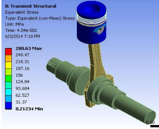
Figure 6: Von mises Stress Plot after Optimization
