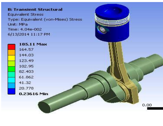
Figure 6: Von mises Stress Plot after Optimization
