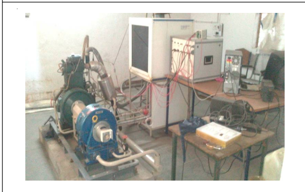
Figure 1: Computerized IC Engine Setup to Obtain P-θ Diagram
