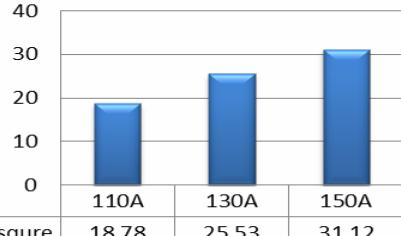
heat. With an increase in welding current, there is a linear increase in arc heat, while the resistance heat increases exponentially which are responsible for electrode melting, resulting increased area of penetration hence dilution.
