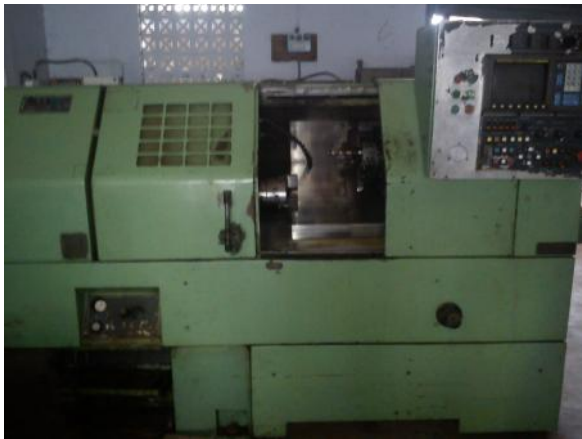
Figure 1: Schublin CNC Machine
