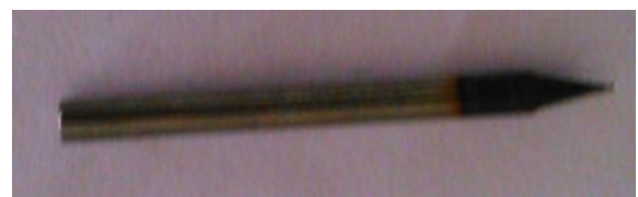
Figure 2: End Mill (Carbide 0.5 mm)
