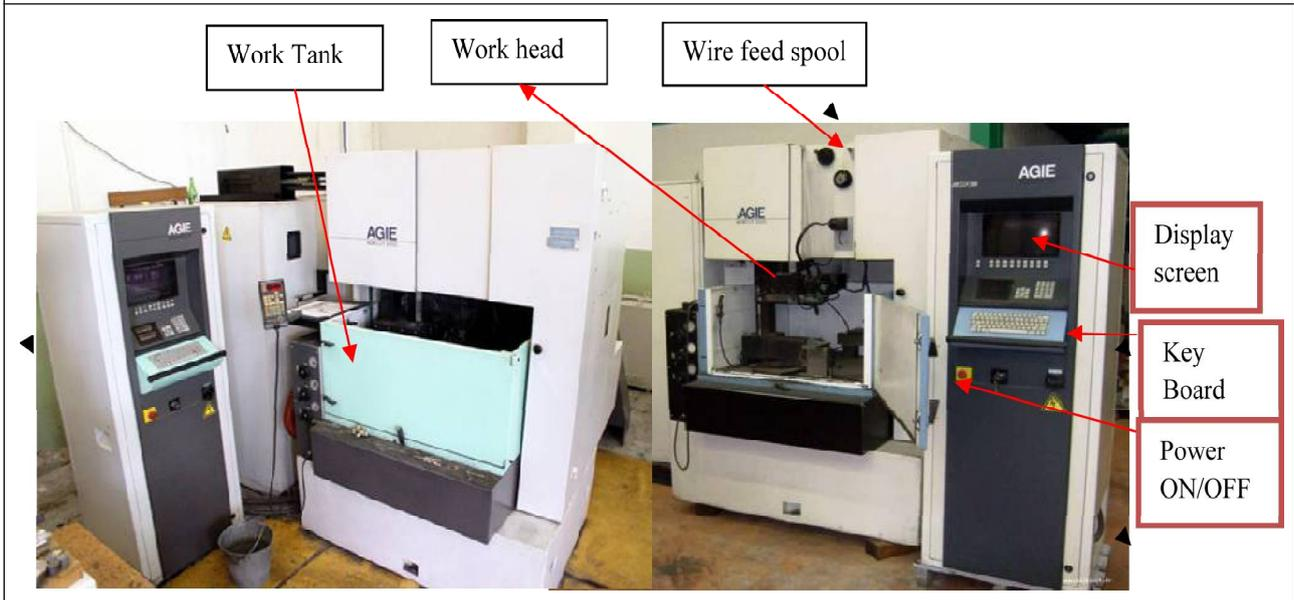
material plate with  $220 \times 40 \times 10$  mm dimensions. Zinc coated brass wire with 0.25 mm diameter and tensile strength of  $900 \text{ N/mm}^2$  was used in the experiments. Average surface roughness ( $R_a$ ) measurements were made by using Phynix
