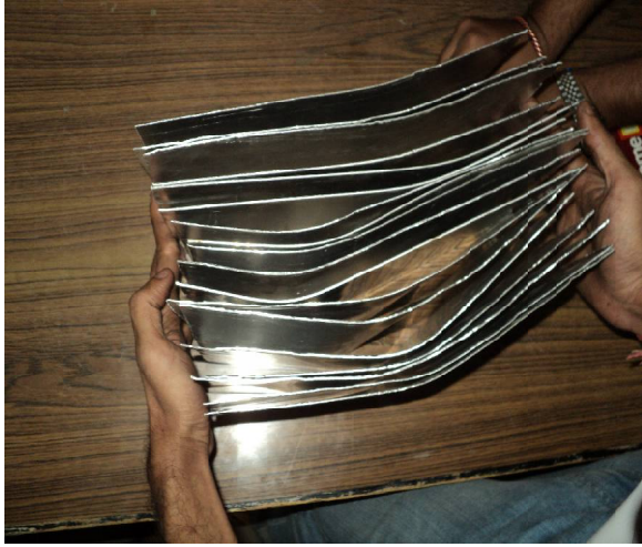
Figure 3: Aluminum Sheet After Deformation
