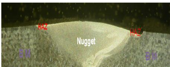
Figure 8a: Weld Cross-Section Macro of AL6063 (at 1400 rpm) and 4 mm / min
