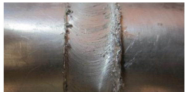
Figure 4: Excessive Weld Flash on Trailing Edge at 485 rpm Speed
