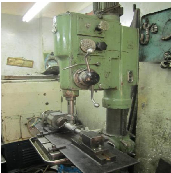
Figure 2: Turn Table and Clamping Device for FSW of Circumferential Weld
