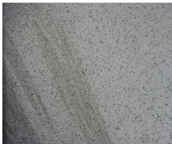
Figure 10a: Image at 200 um Magnification of 6063 Showing the Base Metal, HAZ (at 485 rpm, Feed 4 mm / min)
