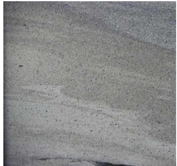
Figure 10b: Image at 200 um Magnification of 6063 Showing Weld Nugget Zone (at 485 rpm, Feed 4 mm / min)
