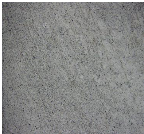
Figure 9a: Image at 200 um Magnification of 6063 Showing the Base Metal, HAZ (at 1400 rpm, Feed 4 mm / min)
