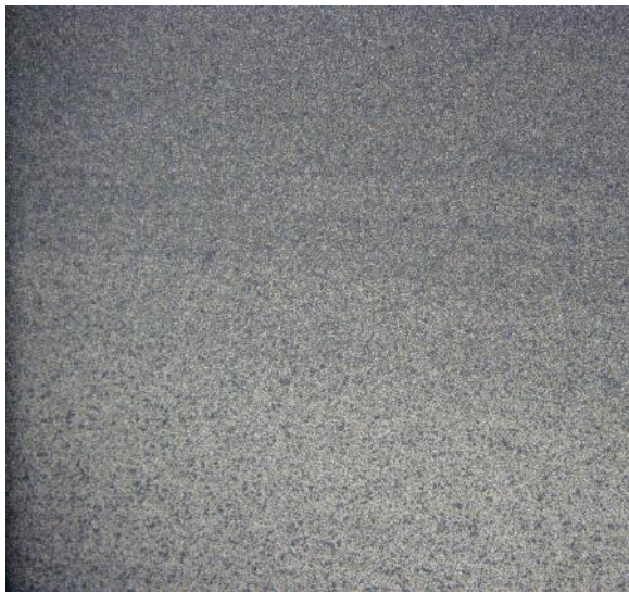
Figure 9b: Image at 200 um Magnification of 6063 Showing Weld Nugget Zone (at 1400 rpm, Feed 4 mm / min)
