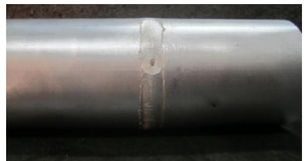
Figure 3: Slight Weld Flash on Trailing Edge that has Exhibited More Good-Quality Welds at 1400 rpm Speed
