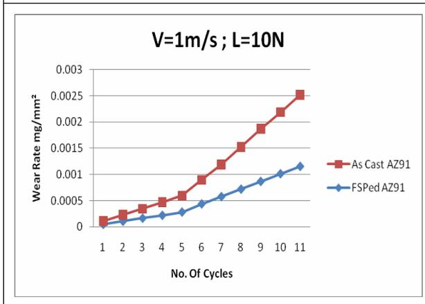
tested for different loads at constant velocity of disc.
