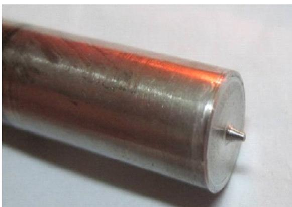
The diameter of the shoulder will determine the amount of contact area applied to the weld material's surface. A shoulder diameter which
