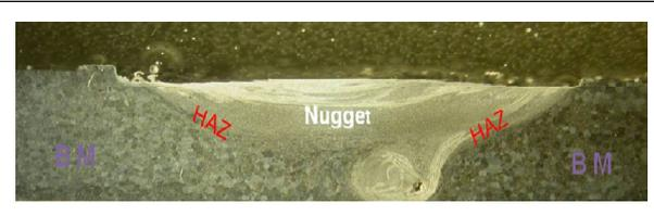
and homogeneous structure obtained, smooth and less porosity surface can be seen in Figure 9 Shrinkage of the pores initiated with 20X in Figure 5.
