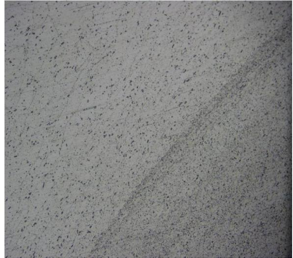
Figures 9 and 10 show the tip of the crack, which is progressing from left to right. It can be seen that the crack is preceded by a large number of voids that formed all the way along the remains of the weld line down to the root of the weld.
