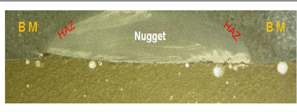
**Figure 8b: Weld Cross-Section Macro of AL6061 Joints Welded at (485 rpm) and 4 mm/min**
