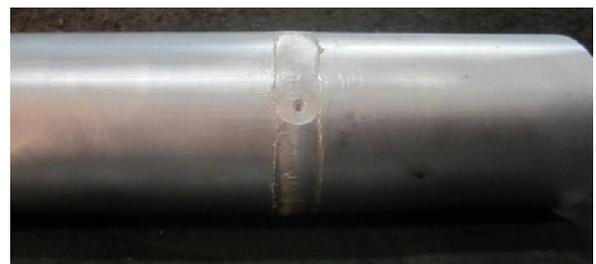
**Figure 4: Excessive Weld Flash on Trailing Edge at 485 rpm Speed**
