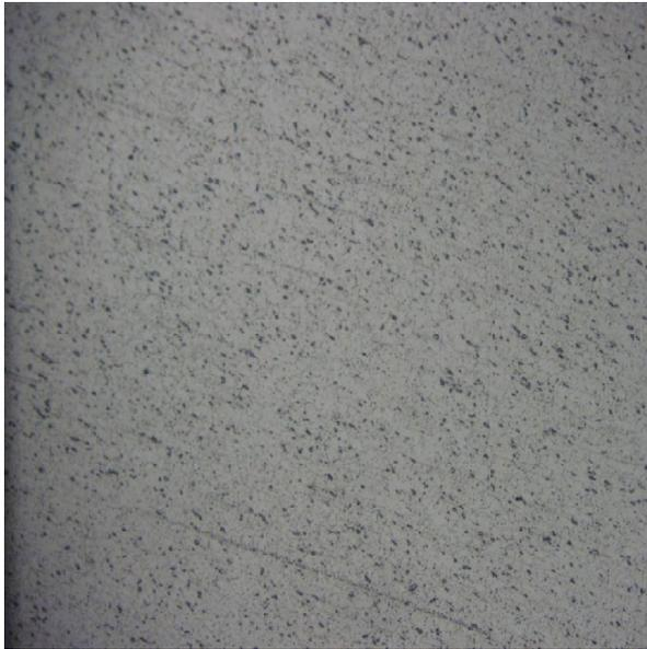
**Figure 10b: Image at 200 um Magnification of 6061 Showing Weld Nugget Zone (at 485 rpm, Feed 4 mm/min)**
