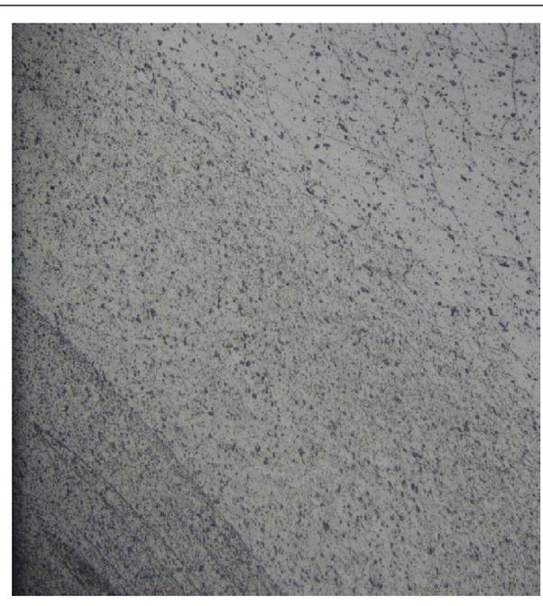
**Figure 9b: Image at 200 um Magnification of 6061 Showing Weld Nugget Zone (at 1400 rpm, Feed 4 mm/min)**
